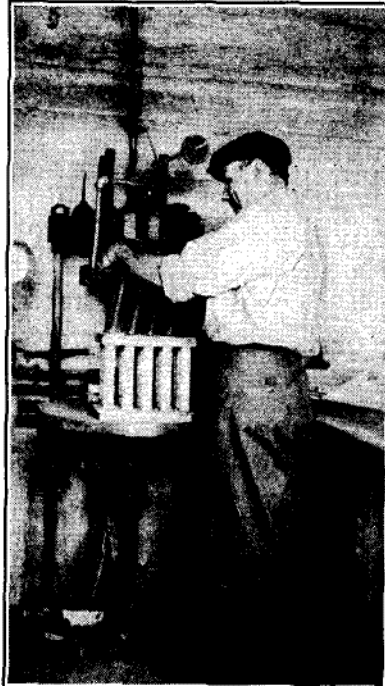
FIGURE 25. Loading Rockets by Means of an Hydraulic Press. (Courtesy National Fireworks Company.)
